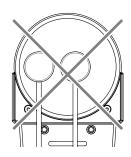
Using a twin pedal will result in lower sensitivity as compared to when a single pedal is used. Raise the sensitivity on the sound module.
